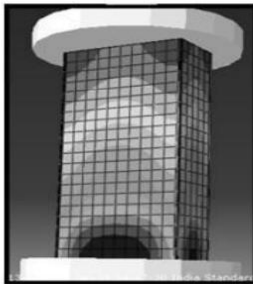
Figure6. Meshed rectangular specimen for computational test
